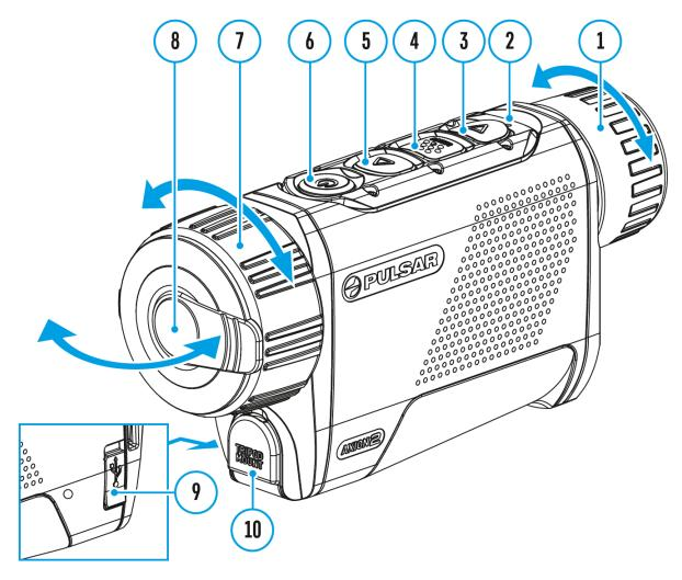
Sensitivity enhancement levels (Normal N), High H), Ultra ()) are software algorithms that enhance the quality of detection and recognition in various observation conditions. When the temperature contrast decreases (fog, precipitation, high humidity), it is recommended to increase the amplification level. To optimize the image, activate the Smoothing Filter in the main menu.
